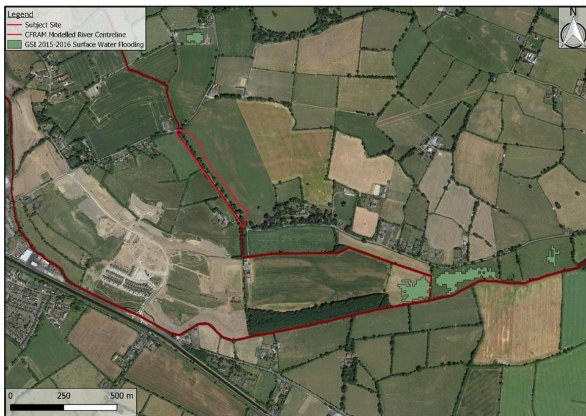
Figure 7-9: GSI 2015-2016 Surface Water Flood Mapping
